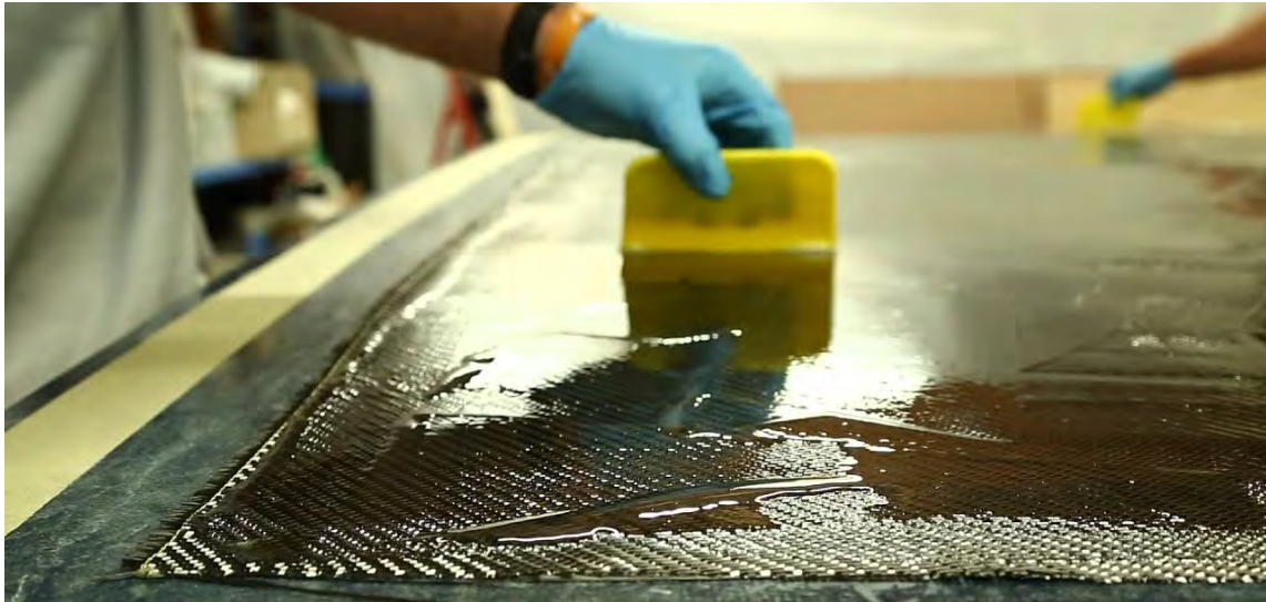
Figure 29: Wet Layup Process
