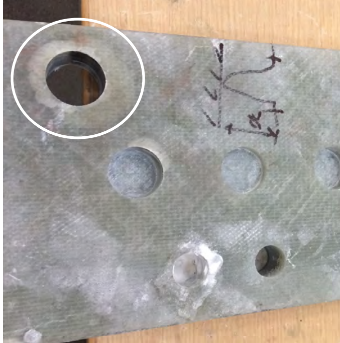
Figure 21: Example of Delamination around a Drilled Hole
