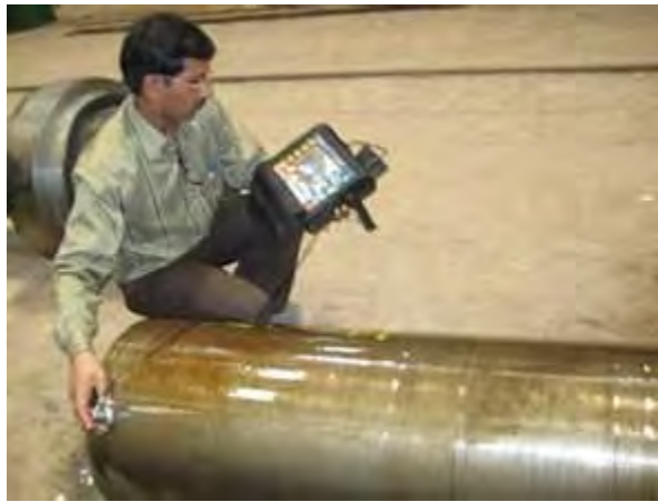
Figure 26 Ultrasonic Testing Equipment with Handheld Transducer and Output Display
